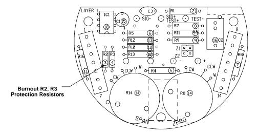
FIGURE 3-4. Compensated Thermocouple Simulator Calibration Diagram.
